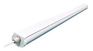
Product wattage: 40W Product Lumen: 6000 Efficiency: 150lm/W CCT: 4000K Body colour: White CRI: 80Ra Lifetime (Hours): 50000 Beam angle: 120° Power factor: 0,9
