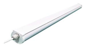
25W Product wattage: Product Lumen: 5400 Efficiency: 150lm/W CCT: 4000K Body colour: White CRI: 80Ra Lifetime (Hours): 50000 Beam angle: 120° Power factor: 0,9
